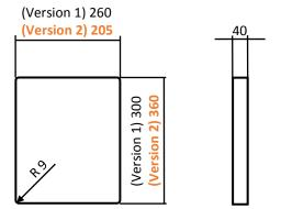
Dimensions version 1: 260 mm x 300 mm x 40 mm **Dimensions version 2:** 205 mm x 360 mm x 40 mm
